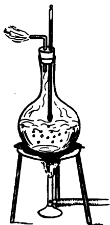
FIG. 8. — Determining one of the fixed points of a thermometer.
